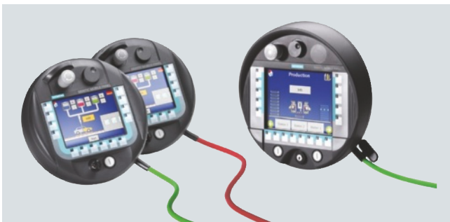
Mobile Panel 177 (left) or 277 (right) – the right model for every application – also with PROFINET/Ethernet connection
